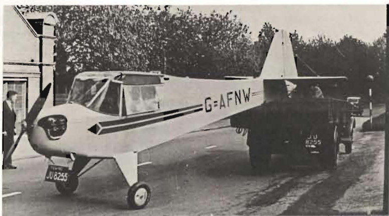
Next stop Ratcliffe ! All aircraft produced by Taylorcraft at Thurmaston were towed to Ratcliffe in this manner for erection and flight. (Leicester Museum of Technology)
